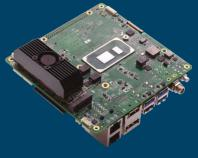
UP AI Core XM 2280 with UP Xtreme i11 Al hardware accelerator with 2x Intel® Movidius™ Myriad X
